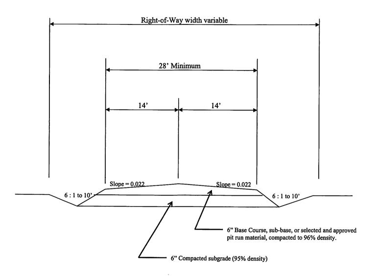
Before beginning preparation of subgrade, all sod and other vegetation shall first be removed from the roadbed to a min. depth of 6".
